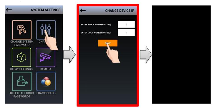
Note: The block number is entered between 01-99 and the door number is entered between 01-19. After entering **THE NEW BLOCK AND DOOR NUMBER** the device becomes re-booth automatically.
