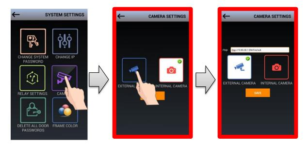
**5.3.4.b INTERNAL CAMERA:** If the internal camera of the door panel will be used **INTERNAL CAMERA** icon is tapped. The device is set to use **INTERNAL CAMERA** as default.
