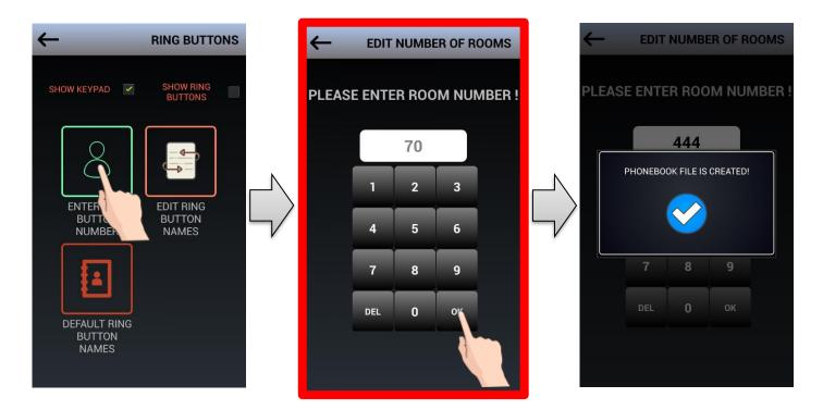
**5.1.6.b EDIT RING BUTTON NAMES:** Names which will be present on the ring buttons are entered via this screen. First enter the room number, then enter the name.
