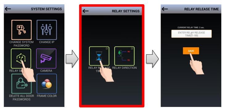
When **RELAY RELEASE TIME** page appears it shows the current relay time and asks to enter the new duration.
