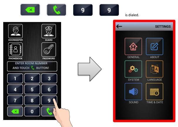
2. Entering SETTINGS if the device screen is button shape: Please press PASSWORD icon LONGER THAN 5 SECONDS.
